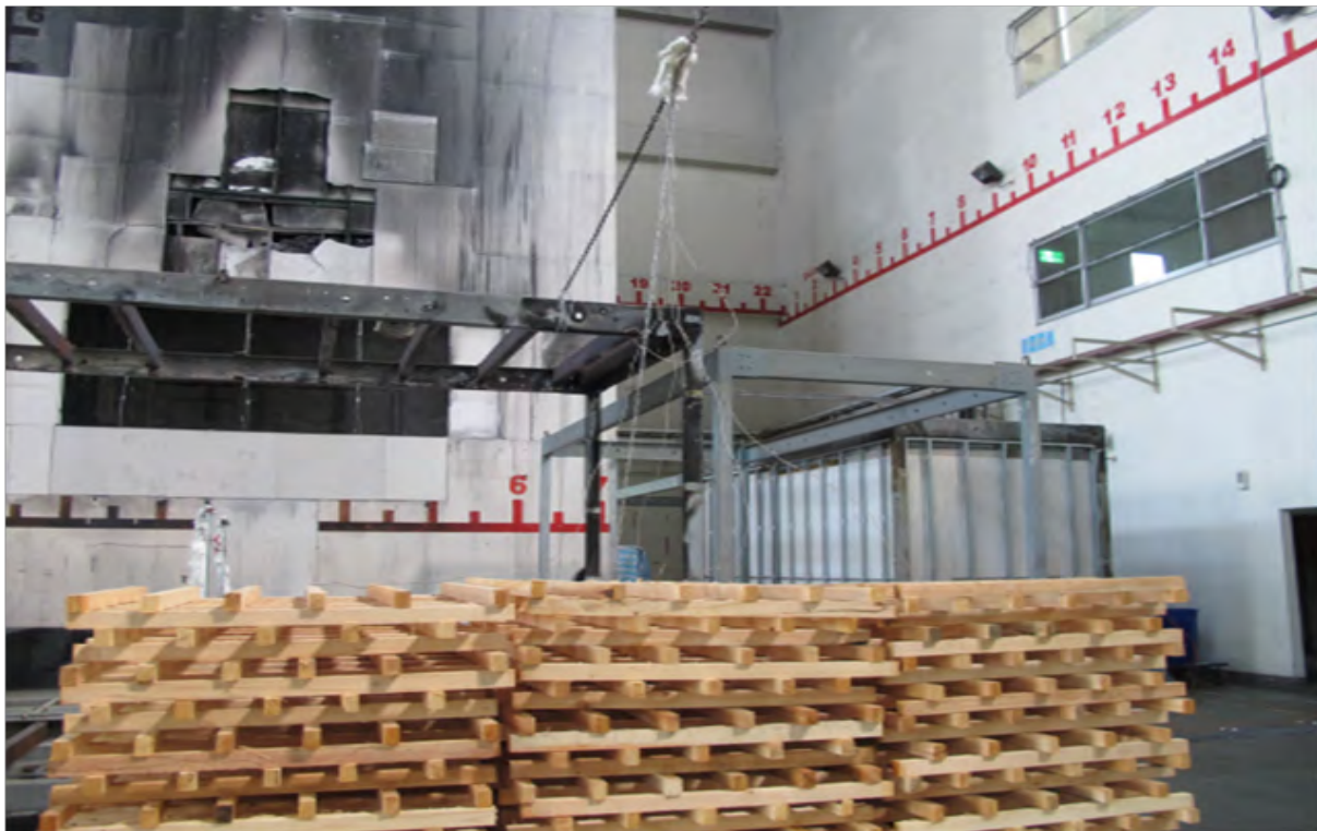
Figure 2. Cross-sectional view of wood cribs and thermocouples
