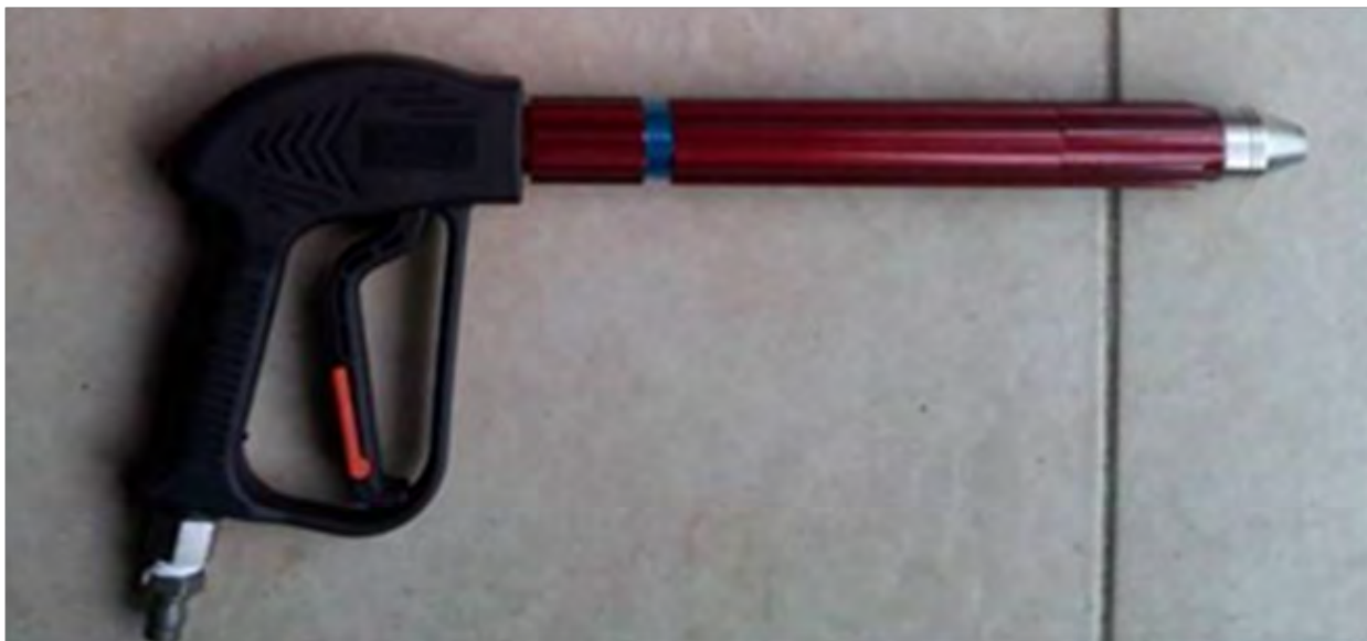
Figure 3. Nozzle A used in the high pressure water mist system.
