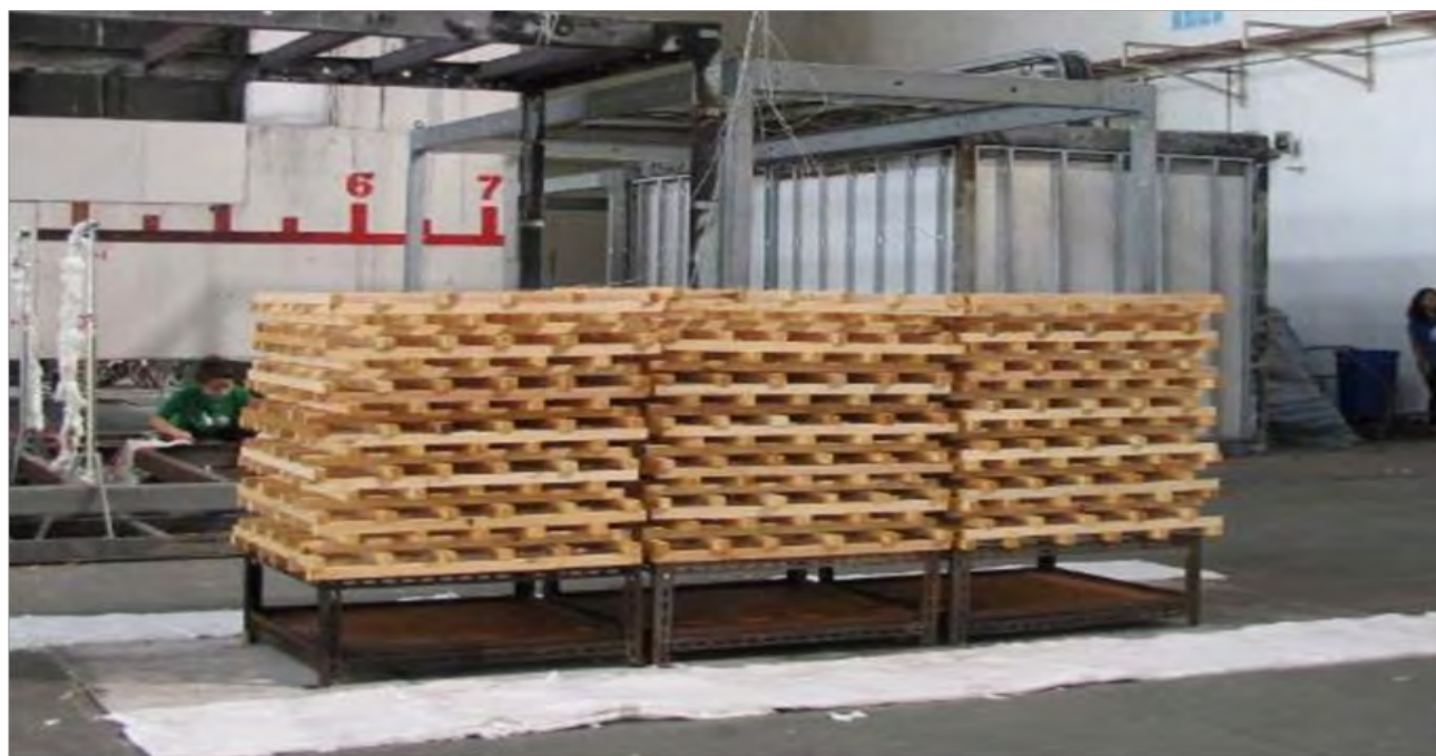
Figure 1. View of three A-2 wood cribs (7.5 MW).
