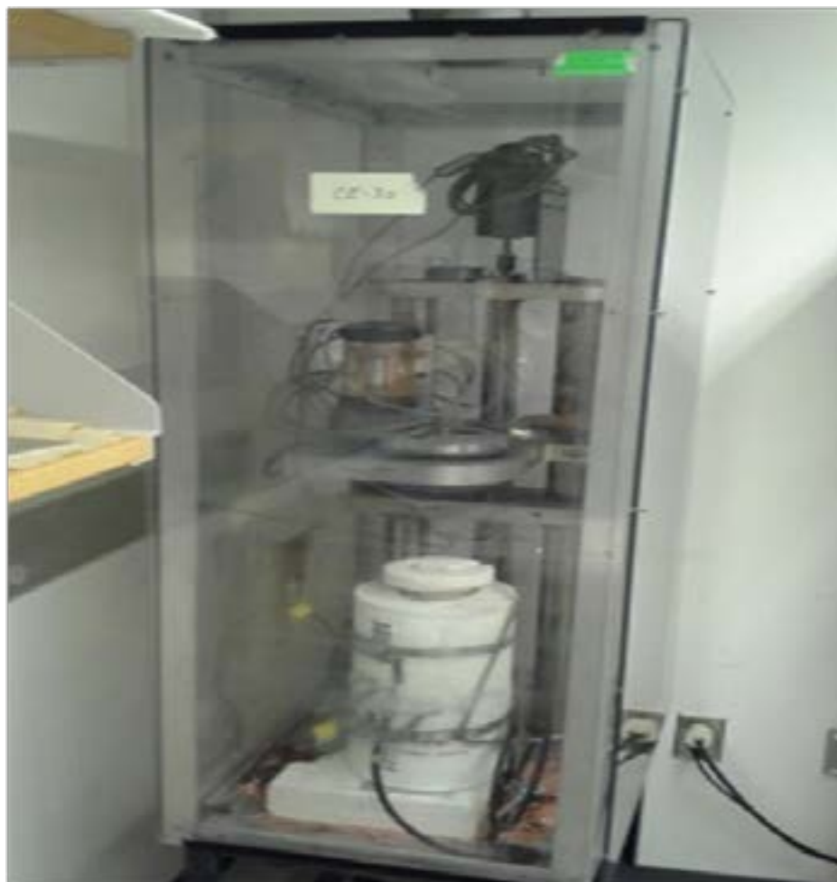
Figure 1. Custom furnace for reactive flux growth containing ceramic insulation and 4 3" diameter thick wall graphite crucible.
