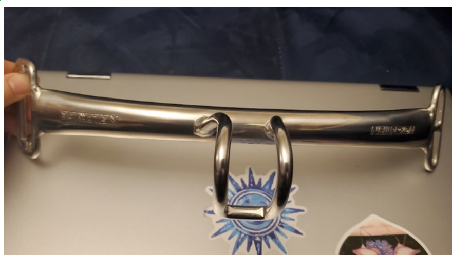
Figure 2: Spreader Bar Used to Distribute Force of the Tow Rope and Allow for Single-Arm Control
