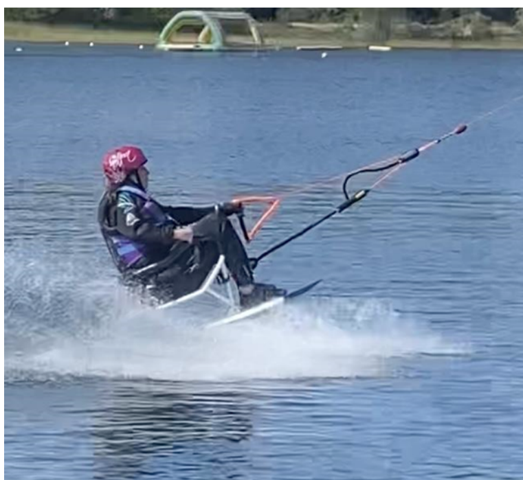
Figure 6: Participant Utilizing the Adaptive Wakeboard System Showing Quick Release Mechanism Attached to Spreader Bar
