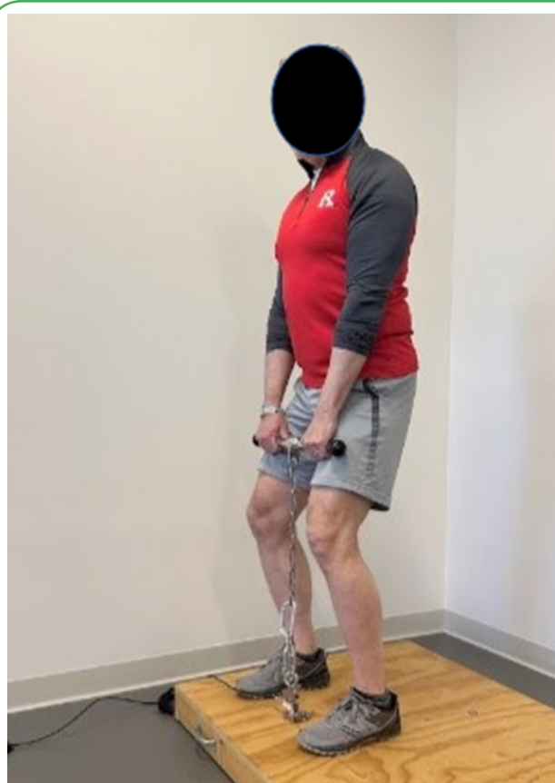
Figure 1. Example set up of IMTP Testing. Participants were positioned with the load cell at the level of the metatarsal heads. Hips and knees were flexed within the acceptable range to position the bar at mid-thigh.
