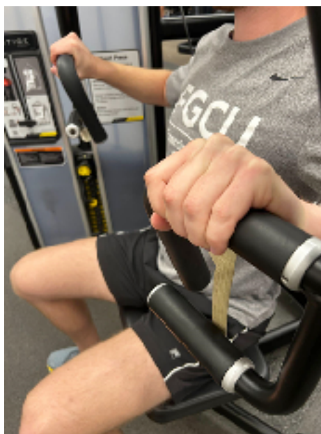
Figure 2. Cybex Chest Press Machine with force pads on the handles
